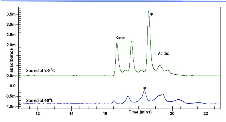
GST electropherogram showing the separation of a 1mg/ml sample the main peak is marked \* and the basic and acidic charge variants are shown.
