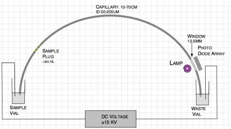
Separations are rapidly performed in a thermally efficient capillary
