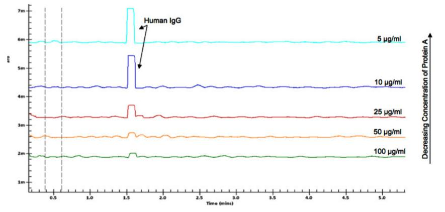
Protein A and IgG were prepared as a mixture in a pH 8 buffer. The concentration of IgG was kept constant at 280  $\mu$ g/ml while the concentration of Protein A was decreased from 100  $\mu$ g/ml to 5  $\mu$ g/ml.
