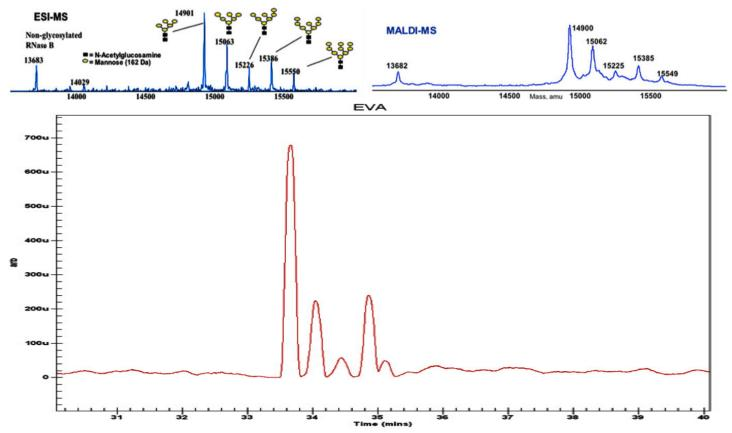
Ribonuclease B Glycoforms can be successfully analysed of HPCE-512 technology comparing favourably to Electron Spray Ionisation MS (ESI-MS \$1M) and MALDI-MS (\$350K).
