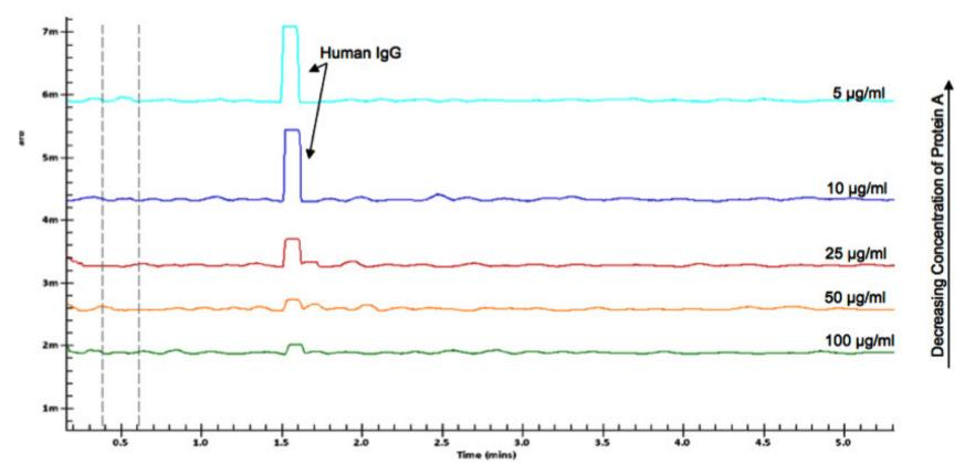
Protein A and IgG were prepared as a mixture in a pH 8 buffer. The concentration of IgG was kept constant at 280 μg/ml while the concentration of Protein A was decreased from 100 μg/ml to 5 μg/ml.
