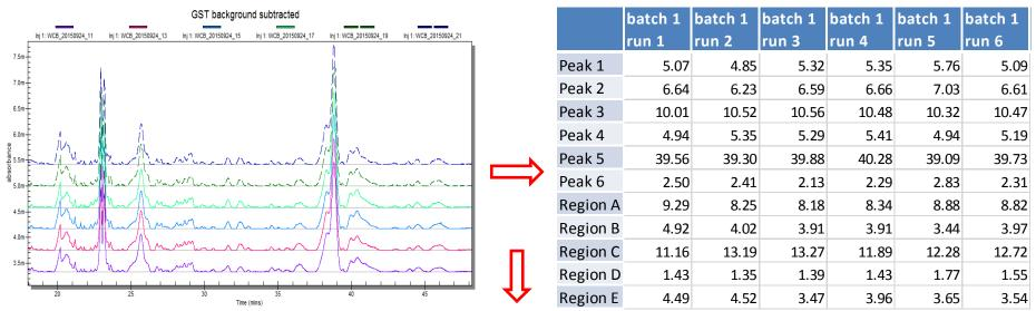
**Step 2**: perform Student's T-test for each quantitative fingerprint region between each pair of sample batches to determine the p-value - the probability of obtaining a result equal to or more extreme than what was actually observed.
