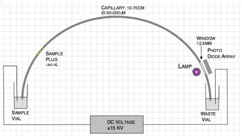
Separations are rapidly performed in a thermally efficient capillary
