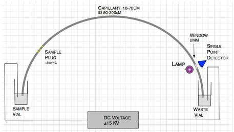
HPCE technology images each analyte band **512** times across a photo diode array at ~**10** times a second.
