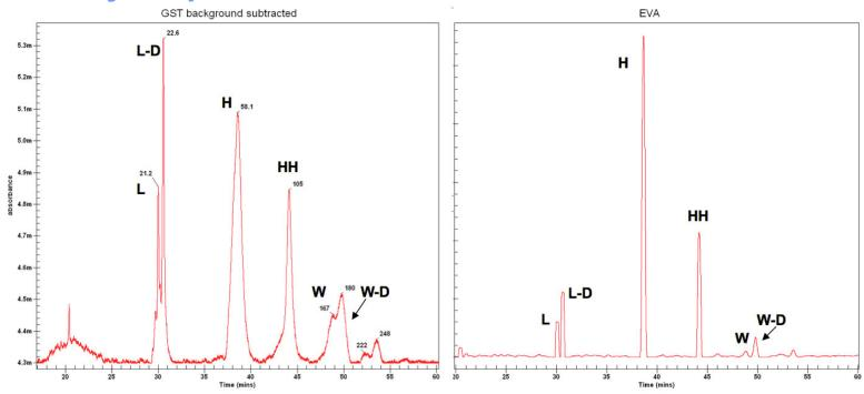
GST electropherogram and EVA trace depicting the separation of non-reduced sample.. Possible assignments have been made for each of the peaks; light chain (L), light chain + drug (L-D), heavy chain (H), heavy-heavy (HH), whole antibody (W), whole antibody + drug molecules (W-D).
