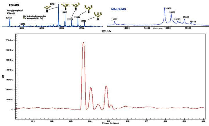
Ribonuclease B Glycoforms can be successfully analysed of HPCE-512 technology comparing favourably to Electron Spray Ionisation MS (ESI-MS \$1M) and MALDI-MS (\$350K).
