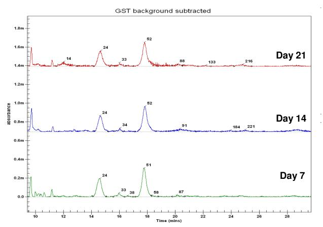
Separation of base treated mAbs. A comparison between the samples analysed at 7, 14 and 21 days is shown. An increased number of very large peaks is observed in the samples analysed on days 14 and 21 compared to the sample analysed on day 7.
