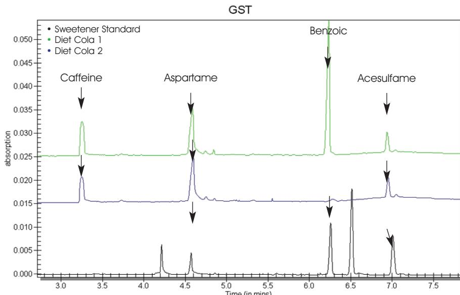
Figure 7: GST electropherograms for standard sweetener and derivatives (black), and Diet Cola 1 (green) and Diet Cola 2 (blue). The caffeine peak at 3.25 minutes was confirmed by separate migration analysis.
